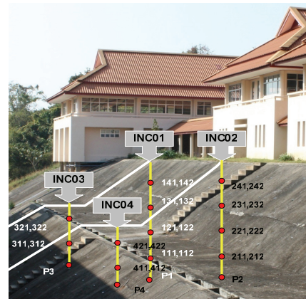
Figure 9: Cross sections and instruments location. (x,y,z) = (position number, sensor number, 1=left side 2=right side)
